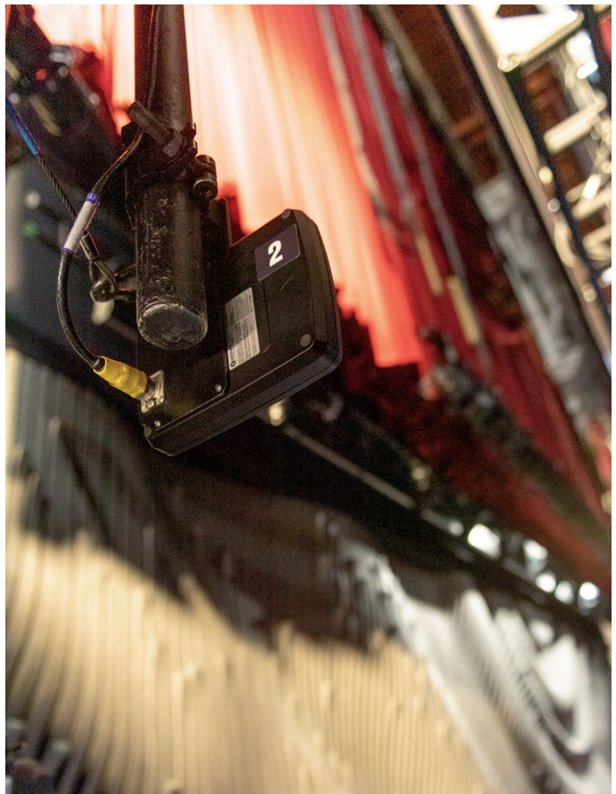
The zackrack tracking system requires at least six antenna elements above the stage
